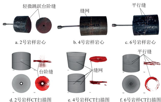
图5 2号、4号、6号试样的压后实物和CT扫描 Fig. 5 Post-fracturing physical samples and CT scans of specimens 2, 4, and 6
